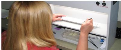
Since 2000 GIA uses low UV emission lamps and diamonds are graded from further away at a pre-set distance.
